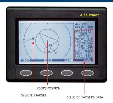
The Automatic Identification System (AIS) is a shipboard broadcast VHF transponder system, sending data about the identity of a ship. Its name, MMSI number, its latitude, longitude, speed, course and heading. All vessels over 300 gross tonnage and all passenger vessels are obliged to carry an AIS transponder. This transponder assists in
