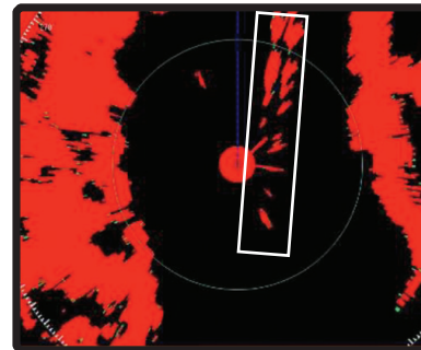
Poles and vessel are less defined on pulse radar display.
