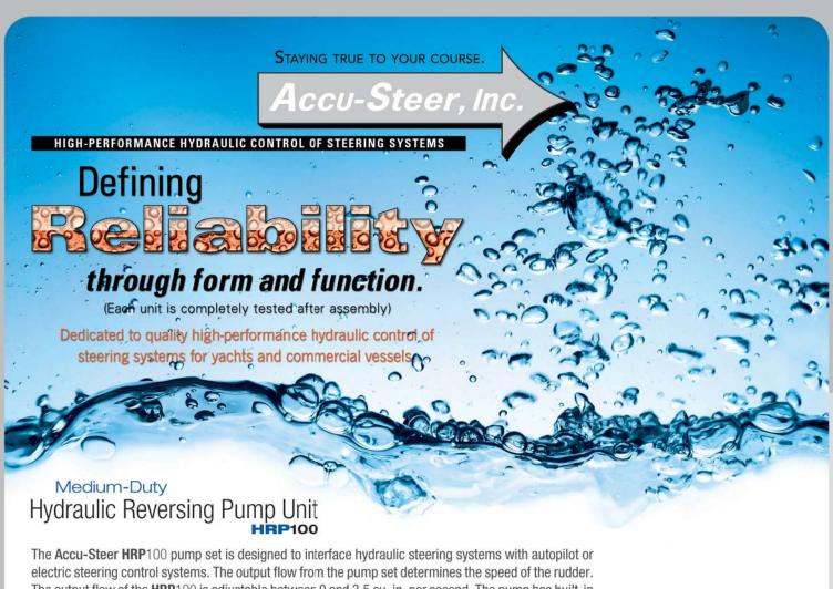
The output flow of the HRP100 is adjustable between 0 and 3.5 cu. in. per second. The pump has built-in pressure relief valves, which are factory set at 500 psi. This pump is recommended for medium-duty applications on hydraulic steering systems that are 50 cu. in. or smaller in volume. The compact and rugged construction provides for easy installation and long life operation. This pump model will interface with most marine autopilot systems. Available in 12 VDC or 24 VDC.
