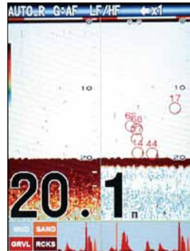
Circles and fish size are displayed on fish echoes. When in dual frequencies mode, you can set the mark displayed on both or either frequency screen.
