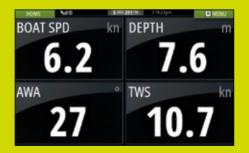
**Instruments** - large instrument display. Connect to your NMEA2000 Network to see data in large, clear digits; the more transducers on the network, the more you will see.
