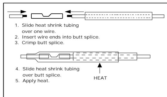
An adequate number of crimp-on connectors and heat-shrink tubing are included with system. The heat-shrink is a special type that will bond to wire insulation and make a watertight connection. See diagram for proper tubing application. Crimp-on connectors are sized for 18 or 20 gauge stranded wire.
