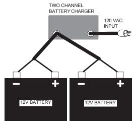
NOTE: If batteries are connected in series for 12/24 - 24V, the series connection wire should be left in place during charging.
