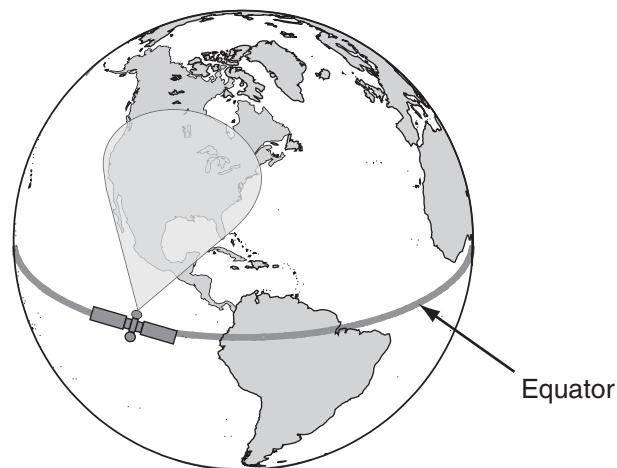
Figure 2-1 Location and Coverage Area of DIRECTV 101 Satellite
