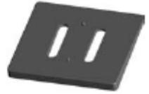
5. Apply a marine sealant to the threads of the two #10 x 1-1/4" self-tapping screws and screw the bracket to the hull. DO NOT tighten the screws completely until you position the transducer as per # 4 above.
