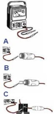
3. Remove the fuse and check for 12 volt power at the spring located inside the fuse housing that is connected to the vessel's power source. If 12 volt power is present continue to the next step. If power is not present, return to Step 1.
