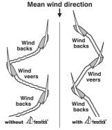
The system automatically calculates the mean wind direction by averaging the true wind direction over a period of time
