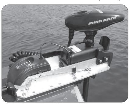
Mount Bracket so that during stow and deploy, the shaft will not encounter boat's rub strip.
