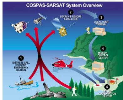
The LUT processes the Doppler-shifted signal from the LEOSAR and determines the location of the beacon, then the LUT relays the position of the distress to a Mission Control Center (MCC) where the distress alert and location information is immediately forwarded to an appropriate Rescue Coordination Center (RCC). The RCC dispatches Search and Rescue (SAR) forces.
