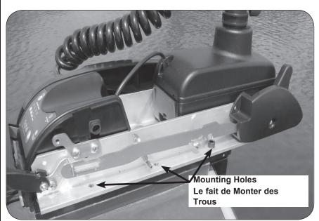
Mount Bracket so that during stow and deploy, the shaft will not encounter boat's rub strip.
