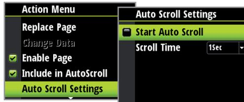
→ **Note:** The scroll time interval can be set to change the displayed data page between 1 and 10 second intervals.
