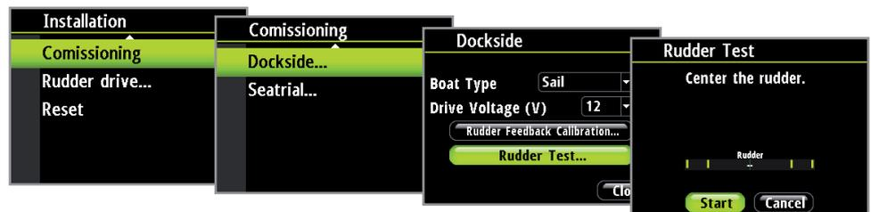
After a few seconds the autopilot Computer will issue a series of PORT and STBD rudder commands and automatically verify correct rudder direction.
