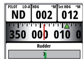
Prior to entering NoDrift mode the autopilot system should be operating in Auto, with valid input from the GPS receiver.
