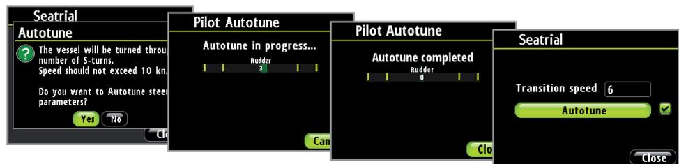
After the Autotune has been completed the rudder must be controlled manually, as the autopilot has returned to Standby mode. The Automatic tuning function will take control of the boat and perform a number of S-turns.
