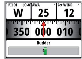
The autopilot will keep the boat on the set wind angle until a new mode is selected or a new wind angle is set.
