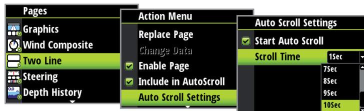
→ **Note:** You can set the time interval of the screen transition from this menu, by selecting Scroll time and modifying the interval time.
