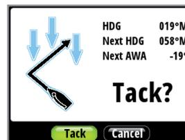
Pressing 'Enter' on the display, or 'Auto' on the Pilot controller, will activate the tack/gybe function and the boat will start turning to the new wind angle.
