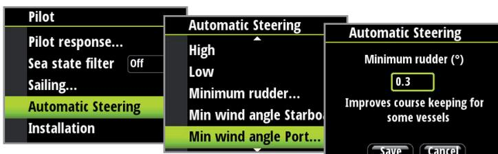
The Minimum wind angle applies for the tack-prevent function. It also applies when the autopilot is operating in WindNAV mode.
