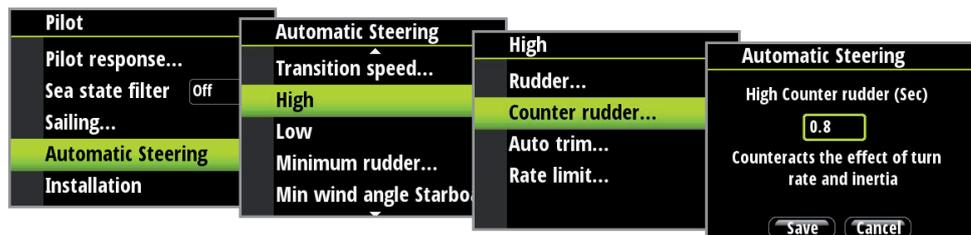
The best way of checking the value of the Counter Rudder setting is when making turns. The figures illustrate the effects of various Counter Rudder settings.
