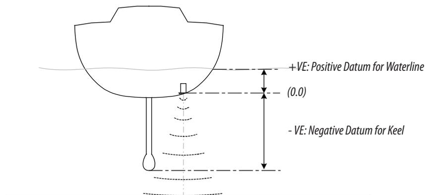
Setting the depth offset displays depth readings from directly below the keel or propellers of the boat, or from the waterline to the seabed. This makes it easier to see the available depth, taking into account the draught of the boat.
