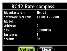
Some devices such as an RC42 compass store their configuration, calibration and offset data in their own memory and not in the display memory. For devices of this type you can check the data information, configure and calibrate the device by selecting Options.
