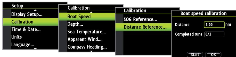
When the boat gets to the predetermined starting position of the distance reference calculation start the calibration timer.
