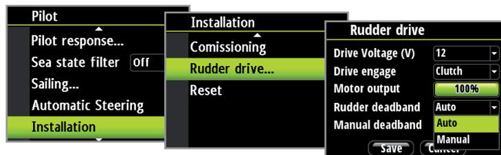
If the auto-setting does not perform properly due to high inertia from the wheel, it can be adjusted manually.
