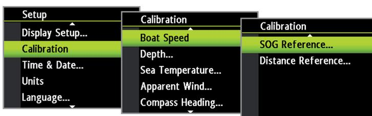
→ **Note:** This calibration should be made in calm sea with no effect from wind or tidal current.
