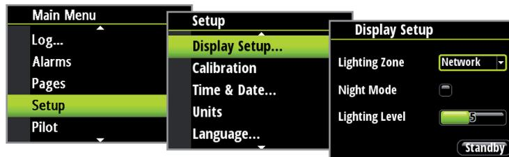
→ **Note:** Press and holding the 'Enter' key for 3 seconds takes you directly to the display setup lighting level screen. If the light level is set below 5 it will automatically increase to 5. Use the up and down keys to set the desired level and press 'Enter' to confirm.
