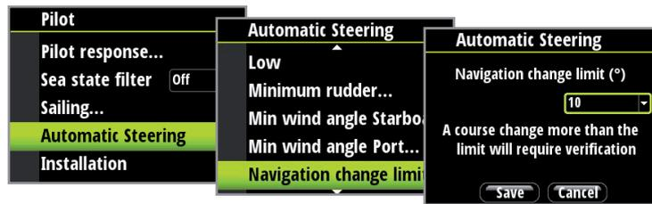
→ **Note:** Nav change limit screen can also be reached from the Nav mode main screen by pressing the 'Menu' key followed by the 'Mode' key within 2 seconds.
