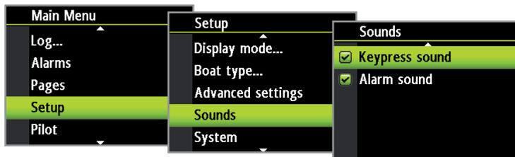
→ **Note:** Silencing the alarm sound does not deactivate the alarms. When an alarm is activated the warning notification will be shown on the display regardless of the sound being on or off.
