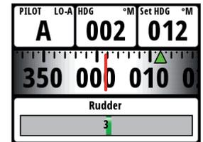
→ **Note:** The autopilot will continue to steer to the set heading until the mode is changed or the autopilot is turned to Standby (disengaged).
