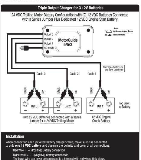
Important: The pair of red and black wires in 1 cable jacket MUST GO TO THE SAME 12VDC battery.
