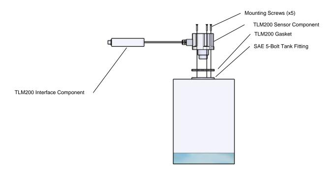
Figure 2 – TLM200 Mounting – SAE 5-Hole Bolt Pattern
