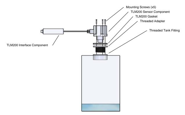
Figure 3 – TLM200 Mounting With Threaded Adapter
