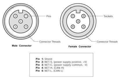
Figure 5 – NMEA 2000<sup>®</sup> Connector Face Views
