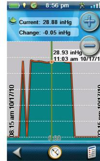
The Barometer Screen (not available on the eXplorist 510) uses the internal sensor in the eXplorist 610 or 710 to graphically display the recorded barometric pressure. The graphic can be zoomed in on, moved, as well as the green line moved along the graphic providing detailed barometric information about the point on the graph selected.
