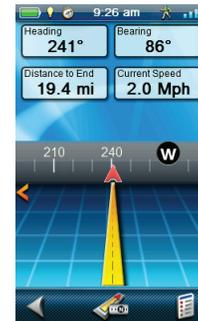
The Road screen displays a graphical road with a strip compass above the road. This compass displays your heading and your heading's relation to the sun, moon and your destination (black arrow) when they are within 50 degrees on either side of your heading. The data fields at the top of the display are customizable (see *Customizing the Data Fields*).
