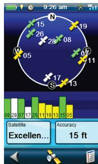
The Satellite Status screen displays a graphical representation of the satellites overhead in relation to you current location (the center of the circle). The color of the satellite graphics, as well as the bar graph, indicate the signal strength of the signals being received. The numbers indicate the assigned satellite designation. The data fields at the bottom of the display are customizable (see *Customizing the Data Fields*).
