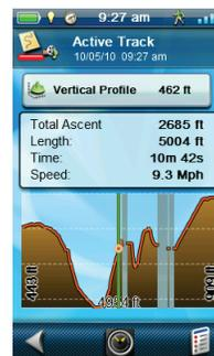
The Altimeter Screen displays detailed elevation information using the GPS signal or the built-in altimeter sensors (eXplorist 610/710). The area on the graph can be expanded by tapping the icon in the lower right corner and defining the area to be used. Also a line can be moved along the graph to pinpoint an exact point on the graph and display detailed information on that point.
