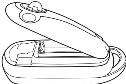
3. Install two AA batteries as shown.
