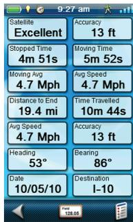
The Data Only Screen displays the most number of data fields available to be viewed at one time in the receiver. Up to 14 customizable data fields can be viewed at one time. The data fields displayed are customizable (see *Customizing the Data Fields*).
