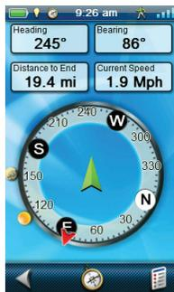
The Compass screen displays a recognizable compass that can be used to display your heading and your heading's relation to the sun, moon and your destination (black arrow). The data fields at the top of the display are customizable (see *Customizing the Data Fields*). The graphic displayed that is used for the compass is customizable as well.
