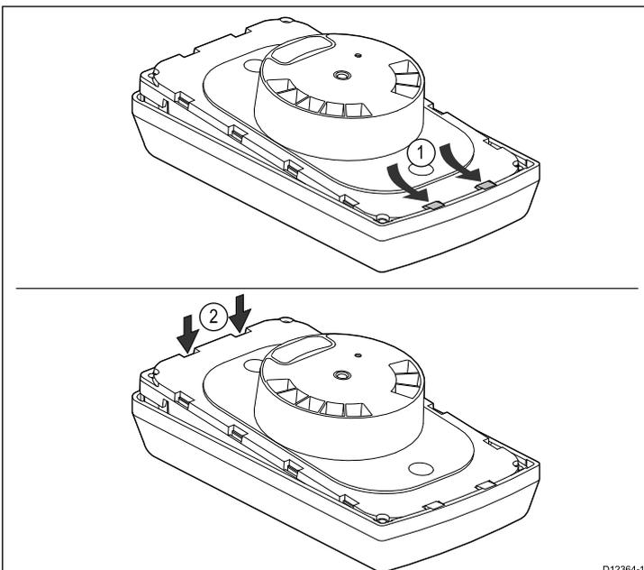
1. Ensure the keymat is positioned correctly.
