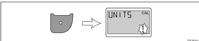
9. Use the **Up** and **Down** buttons to select the required speed units.
