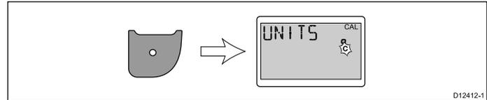
13. Use the **Up** and **Down** buttons to select the required temperature units.
