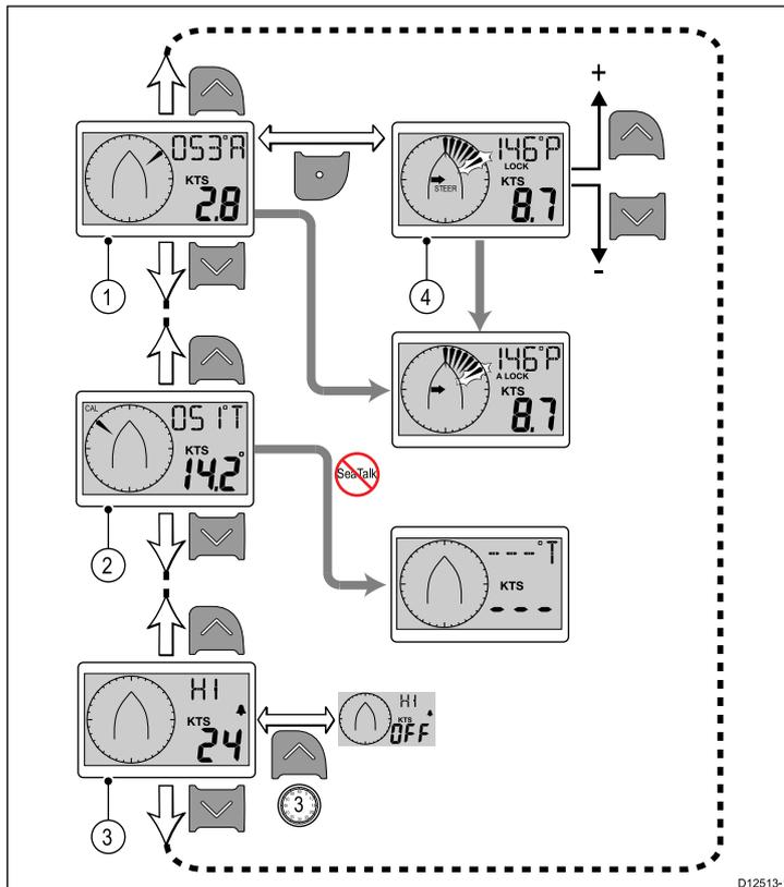
**Note:** The **High wind speed alarm** page is only available on master units (See the *Data master* section for details), it is a temporary page which will time out after 5 seconds to the previous permanent page.
