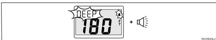
The Deep alarm is available on both the i40 Bidata and i40 Depth instruments. The Deep alarm sounds when the depth is equal to the Deep alarm threshold. The alarm sounds until silenced manually.
