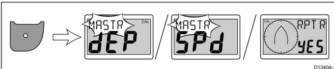
**Note:** The i40 Bidata requires an extra Action button push to switch from depth instrument status and speed instrument status.
