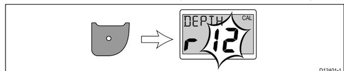
3. Use the **Up** and **Down** buttons to adjust the depth response to the required level.
