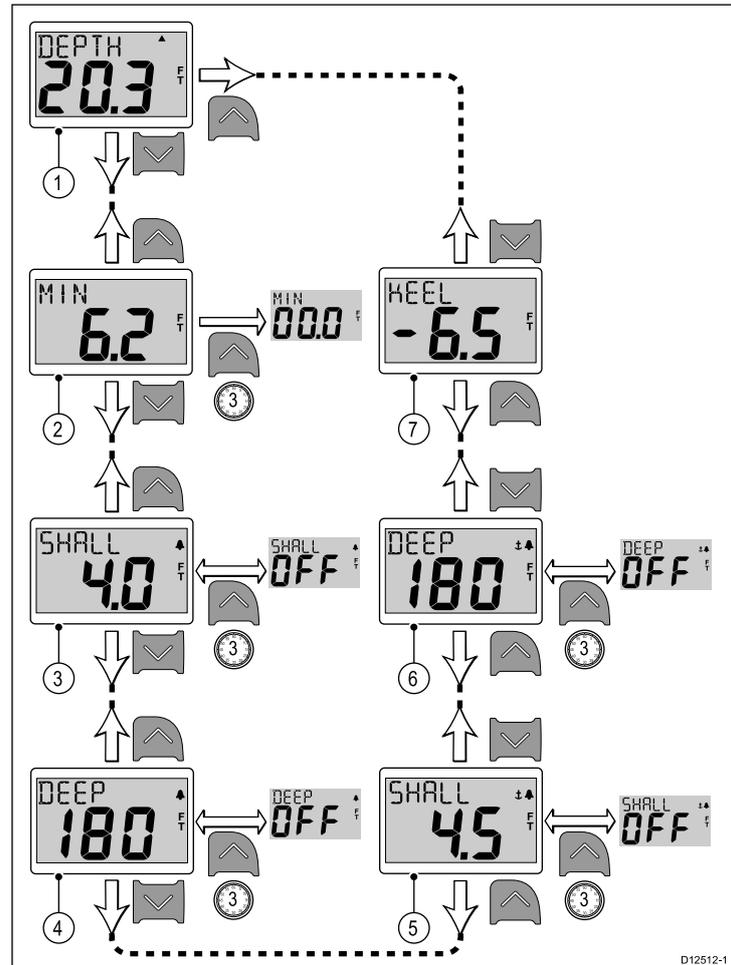
**Note:** Alarm and offset pages are only available if the unit's status is set to Master (See the *Data master* section for details).
