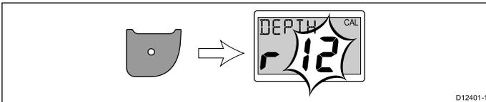
3. Use the **Up** and **Down** buttons to adjust the depth response to the required level.
