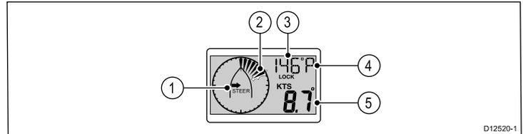
**Note:** If **A LOCK** is displayed the wind angle is controlled by the course computer and cannot be changed manually.
