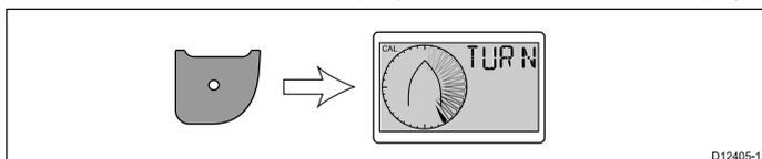
**Note:** If 5pd is displayed on the linearize transducer page the wind speed is outside of the range suitable for linearization.
