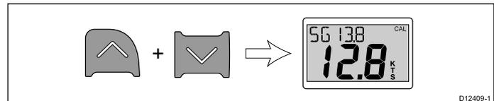
The SOG page is only displayed if SOG data is available and the vessel speed is greater than 0.5 kts.
