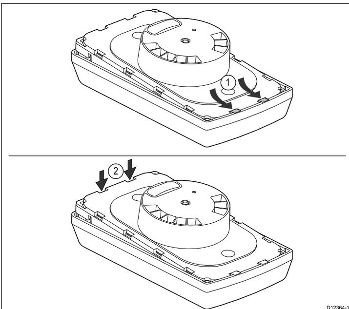
1. Ensure the keymat is positioned correctly.
