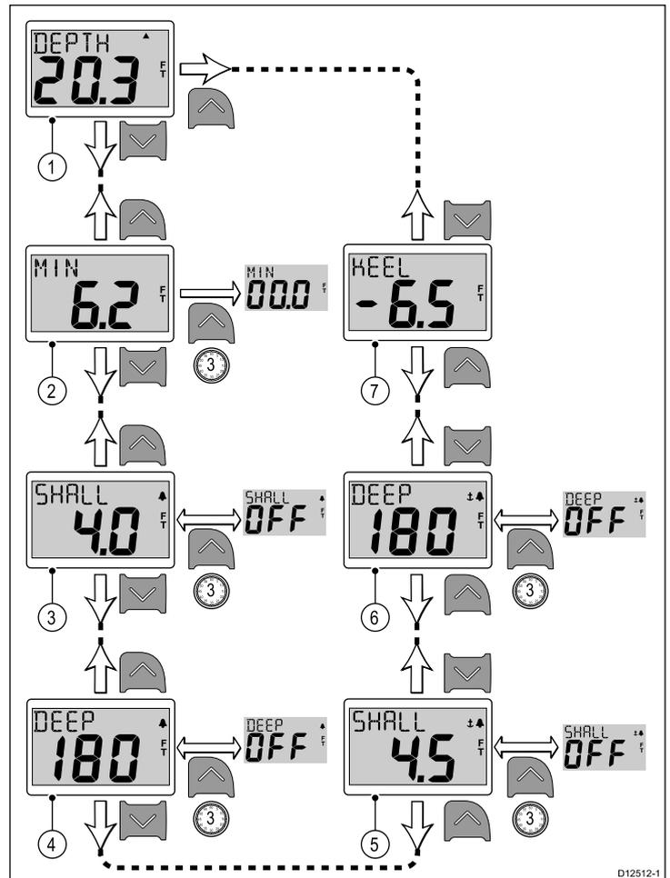
**Note:** Alarm and offset pages are only available if the unit's status is set to Master (See the *Data master* section for details).
