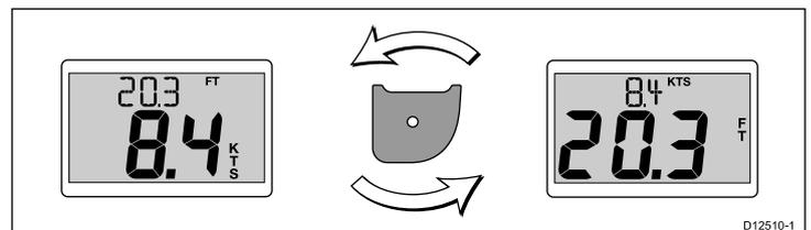
1. Press the **Action** button to switch speed and depth positions on the display.
