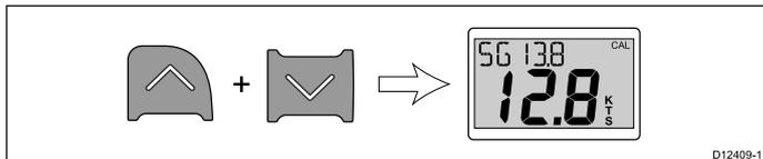
The SOG page is only displayed if SOG data is available and the vessel speed is greater than 0.5 kts.
