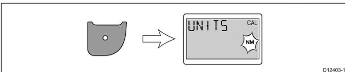
11. Use the **Up** and **Down** buttons to select the required distance units.
