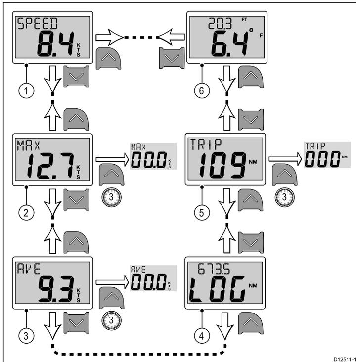
**Note:** The trip distance reading can only be reset if the unit's status is set to Master (See the *Data master* section for details).
