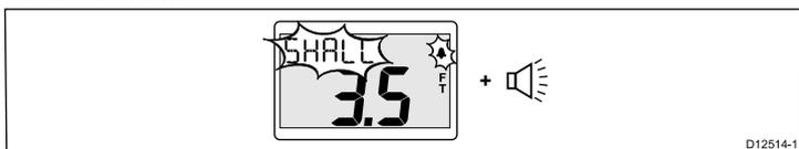
The Shallow alarm is available on both the i40 Bidata and i40 Depth instruments. The Shallow alarm sounds when the depth is equal to or less than the Shallow alarm threshold. The alarm sounds until silenced manually.
