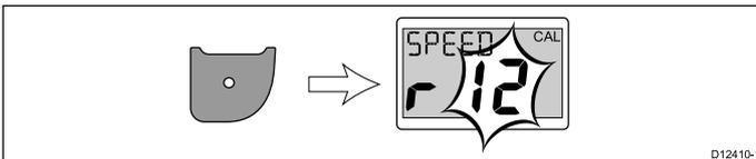
5. Use the **Up** and **Down** buttons to adjust the speed response to the required level.
