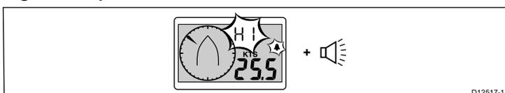
The High wind speed alarm is available on the i40 Wind instrument. The High wind speed alarm sounds when the wind speed exceeds the High wind speed alarm threshold. The alarm sounds until silenced manually.
