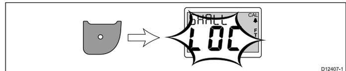
21. Use the **Up** and **Down** buttons to switch the shallow alarm lock on and off.
