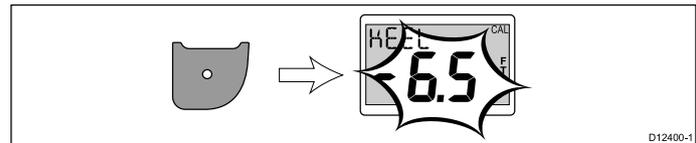
19. Use the **Up** and **Down** buttons to select the required depth offset value.
