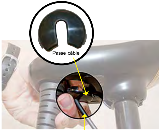
FIGURE 15 Sonar Cable (Universal Sonar Motors Only)
