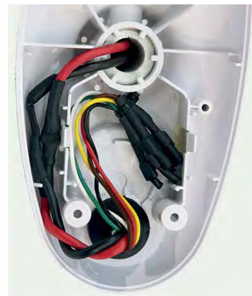
FIGURE 21 Place insulated AutoPilot wires in the bottom center of the control box as shown.
