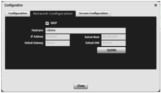
Figure 13 – Configuration Dialog, Network Tab
