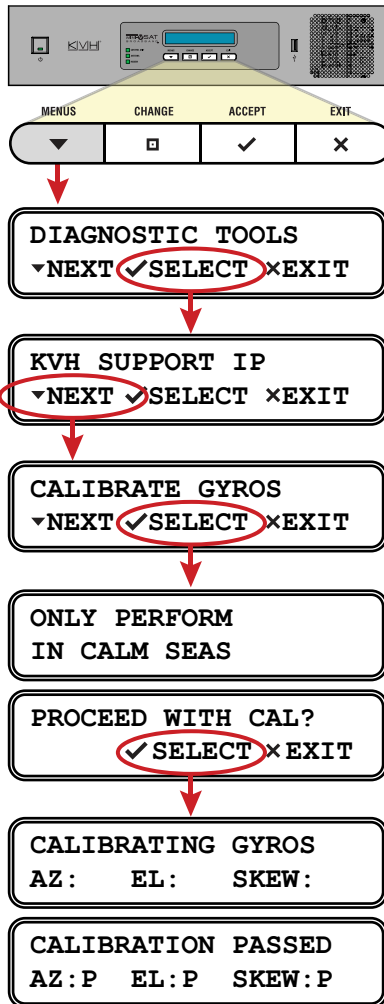
Figure 9-13 Calibrating the Gyros
