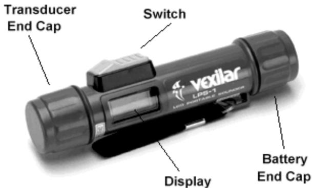
Place the transducer end of the unit in the water, make sure you are pointing straight towards your target. For example, straight down towards the bottom. The LPS-1 will continue to monitor the depth as long as the switch is held in the forward position. When the switch is released the depth reading will stay locked
