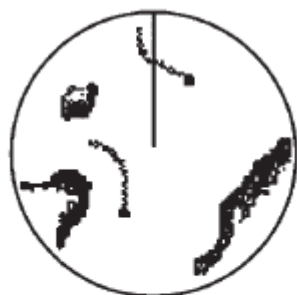
(a) True target trails (No smearing of stationary targets)
