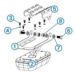
2 Attach the transducer mount bracket to the trolling mount bracket (§) using the included 16 mm M8 bolts (§), M8 flat washers (?), and M8 lock nuts (§).
