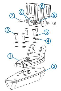
2 Secure the mount to the bracket (6) with the included 12 mm M4 screws ⑦, M4 flat washers (8), and M4 lock nuts (9).
