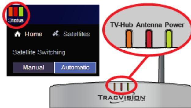
During normal operation, all three lights should be lit green. The following tables explain what the different light conditions indicate. If an error condition exists, view the error message on the Home page of the web interface (see [“Error Messages”](#) on page 90).
