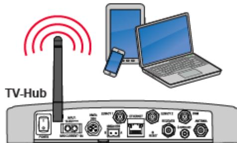
*NOTE: This direct wireless connection will not work if you changed the TV-Hub's wireless settings from Access Point mode to Infrastructure.*
