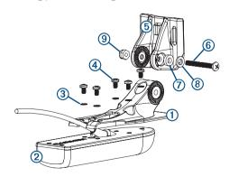
2 Attach the mount to the bracket ⑤ with the bolt ⑥, rubber washer ⑦, flat washer ⑧, and lock nut ⑨.
