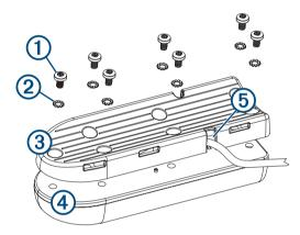
**2** Route the cable through the cable exit ⑤ so the cable is on the top side of the trolling motor housing when stowed.
