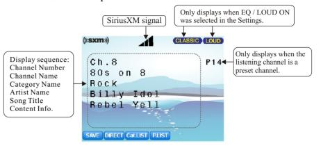
SAVE: To save current channel into P.List. DIRECT: To directly input a channel No. Cat.List: To display the Category List. P.LIST: To display the Global Preset List.
