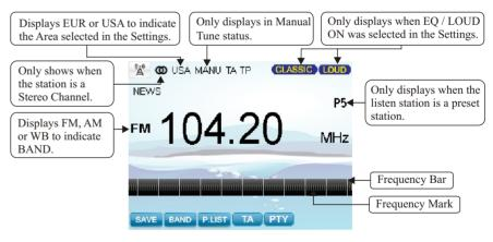
SAVE: To save current frequency into P.List BAND: To select FM, AM or WB band
