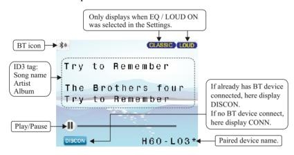
CONN: To establish Bluetooth connection. DISCON: To disconnect the BT Device.
