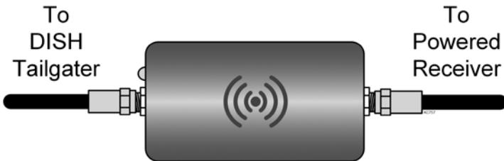
The KING AL1000 Alarm goes in-line between your powered receiver and the DISH Tailgater.
