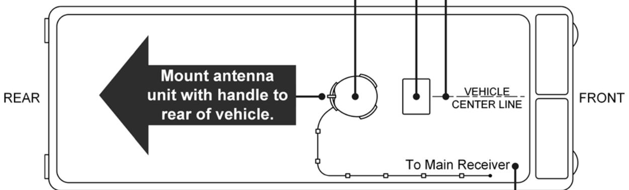
**Mount antenna unit with handle to rear of vehicle.**
