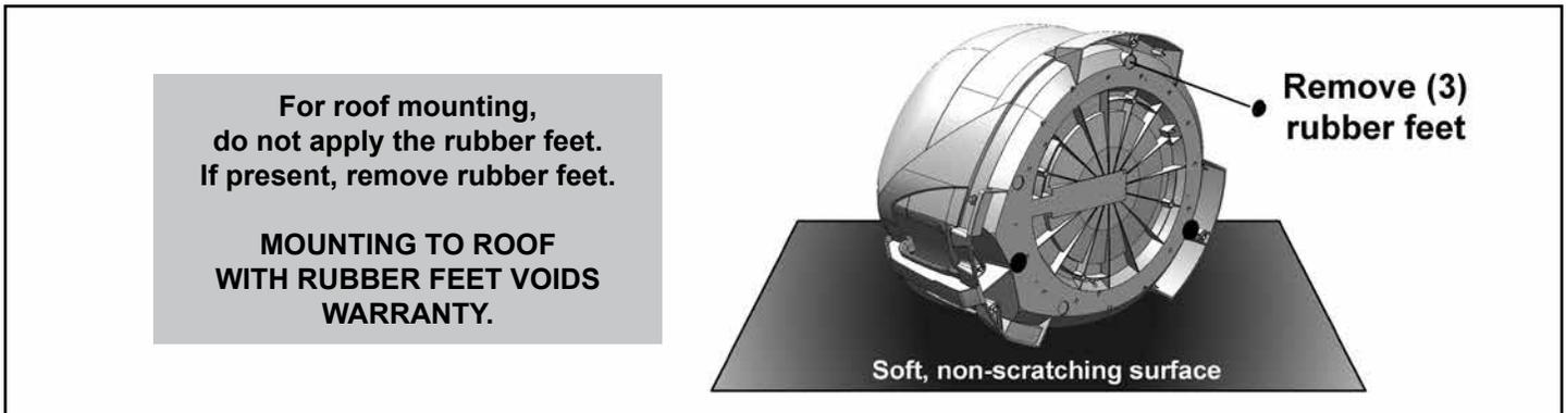
4. Mount the antenna unit using the (4) mounting holes. Make sure to seal mounting holes with roof-compatible sealant. **DO NOT BLOCK THE (5) DRAIN HOLES WITH SEALANT.**
