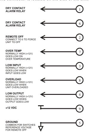
Note: All switches are electronic (solid state) not mechanical relays.
