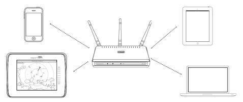
The WatchMate can also join an existing network. It can do this in either DHCP mode (default) or you can set a static IP address. To prevent the address from automatically changing we recommend that you use a static IP address.
