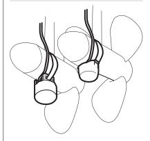
NOTE: The transducers shown below have a directional bias, and therefore need to be oriented according to the illustration below.
