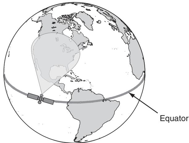
In addition, since TV satellites are located above the equator, the TracVision antenna must have a clear view of the sky to receive satellite TV signals. Anything that stands between the antenna and the satellite can block the signal, resulting in lost reception. Common causes of blockage include boat masts, trees, buildings, and bridges. Heavy rain, ice, or snow might also temporarily interrupt satellite signals.
