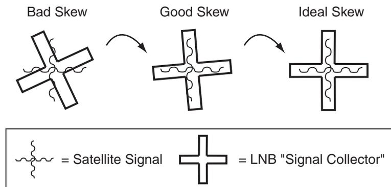
The correct skew setting varies depending on your geographic location, since the orientation of your antenna to the satellite changes as you move. For example, if your antenna is tracking the PAS 9 satellite for Sky Mexico programming, the ideal skew setting ranges from +30 to +70, depending upon your location within the satellite's coverage area (see Figure 1-4).
