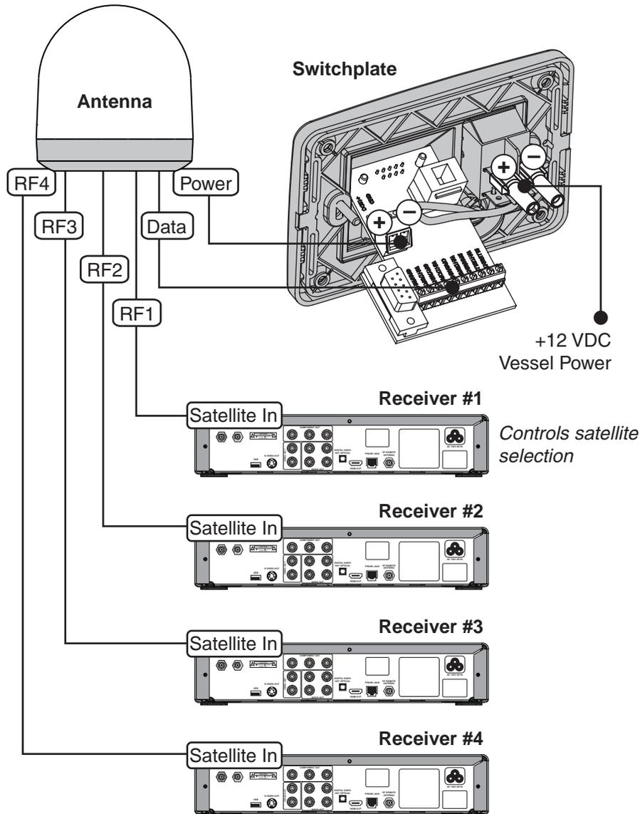
**\*NOTE:** If you wish to connect more than four receivers, you will need to install an active (powered) multiswitch, such as Spaun model SMS5602 NF (KVH Part #19-0413). Multiswitch configurations require the use of either a PC, an optional TV/SAT Switch (KVH Part #01-0245), or a MultiSat Control Panel (MCP) (KVH Part #01-0260-02) to switch between satellites.
