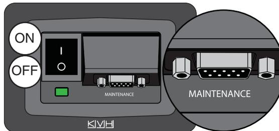
2. Connect a serial data cable from the maintenance port (DB9 connector) located on the switchplate to the serial port on your PC.
