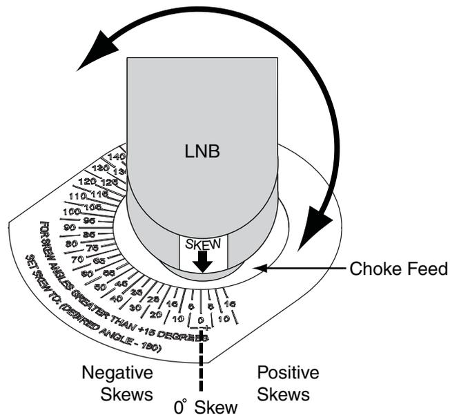
**5b. TracVision M7 Only** - Adjust the LNB clockwise or counter-clockwise, until the skew arrow on the LNB points to the skew angle that you determined earlier.
