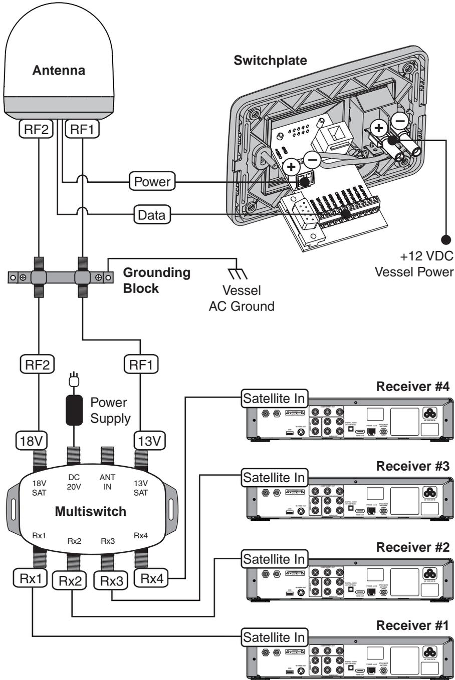
**\*NOTE:** This configuration does not support automatic satellite switching. This configuration requires an Eagle Aspen multiswitch (KVH Part #72-0310). This configuration also requires a PC, an optional TV/SAT Switch (KVH Part #01-0245), or a MultiSat Control Panel (MCP) (KVH Part #01-0260-02) to manually switch between satellites.
