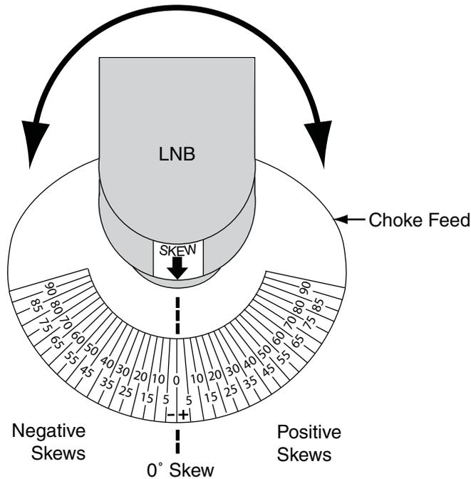
6. Tighten the two M4 socket set screws to secure the LNB in place. Apply 9 in-lbs (1 Nm) of torque, if possible.
