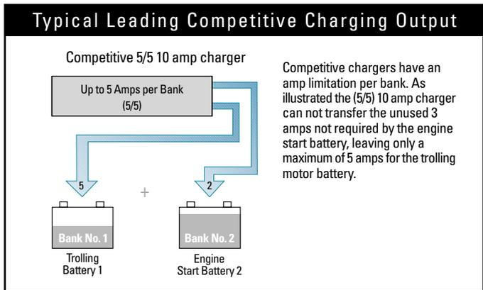
Above illustration reflects typical battery usage after a day of fishing. Trolling motor batteries are 50% discharged and not usable. Engine start battery is 90% charged from the engine charging system.
