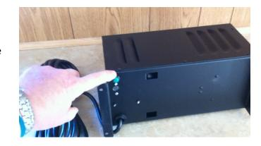
Spray the Temperature Sensor 2-3 short blasts with the Freeze Spray. The heater will come on indicating normal operation. If the ambient air is above 40 degrees the heater will cycle off after a few minutes.
