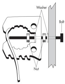
To mount the jack, hold it parallel to the three clamps. Put one end of the jack into a Quick Fist clamp, with the bolt through the steel bar, then lock the clamp loosely. Next, place the steel bar into the other two clamps and lock. After all three clamps are holding the jack, tighten as necessary.
