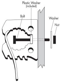
For certain applications, such as roof racks with round tubing, you can install Quick Fists using hose clamps. Make sure you center the hose clamp on Quick Fist's plastic washer to avoid cutting into the rubber clamp.
