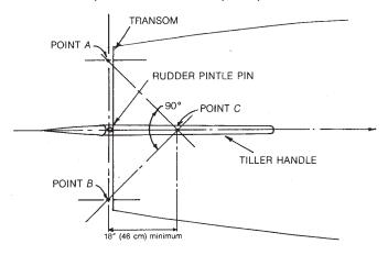
3. Assemble the Tiller-Tamer unit to the tiller handle by positioning the knob over point C. Attach with two wood screws provided. Release the knob and thread the 1/4" (6.4 mm) line through as shown below.
