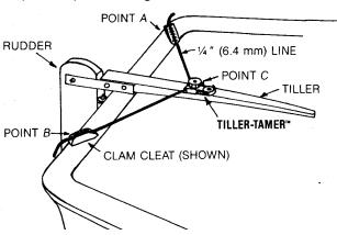
**4.** Attach a cleat at points A and B. This may be a clam cleat or any other quick releasing device. CL201 is recommended, as shown above.
