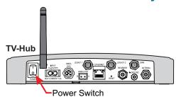
At the rear panel of the TV-Hub, set the power switch to the On position. The TV-Hub supplies power to the antenna. Wait a few minutes for system startup.
