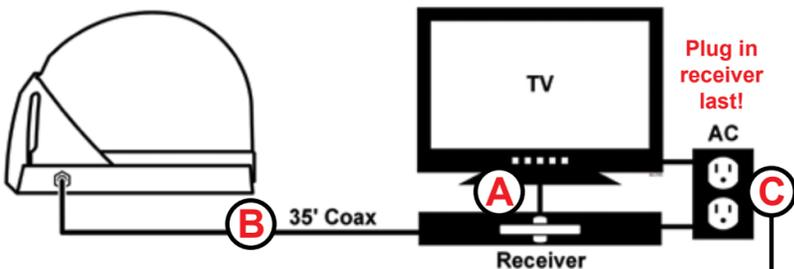
**Do not over tighten coax connections! Do not pull on coax.**
