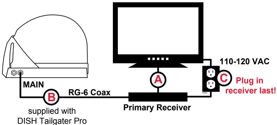
**Do not overtighten coax connections!**
