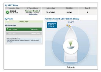
Connect to the vessel's network (the same network to which the ICM is connected). Then start your web browser and enter http://minivsat.kvh. If this doesn't work, enter the ICM's IP address (default is 192.168.5.1). You can find this address on the LCD: go to Settings > Network Settings > IP Assignments.
