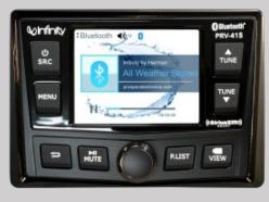
marine digital media receiver •works with your boat's NMEA 2000 system works with SiriusXM's satellite radio tuner •RGB Control with MIL-LEDPWR box compact design fits into standard gauge openings
