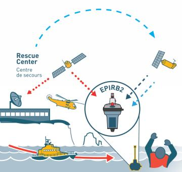
Harnessing the global reach of the Cospas-Sarsat Satellite Network, the EPIRB2 can be activated anywhere, at any time, and will transmit your 406 MHz distress message. The distress transmission includes beacon coordinates that are derived from the EPIRB's integrated GNSS receiver and are accurate to within 100 meters.
