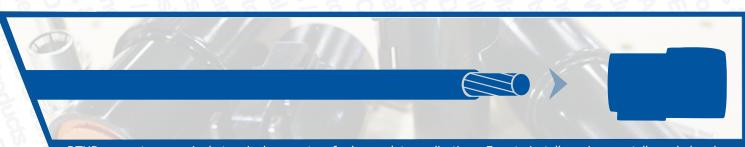
DTHD connectors are single terminal connectors for heavy duty applications. Easy to install, environmentally sealed and compact in size, they are a simple, field serviceable alternative to a splice. Pacer assembled power connector kits that contain a plug & socket with a receptacle & pin to create a sealed power connection for wire guages 10-6 AWG.
