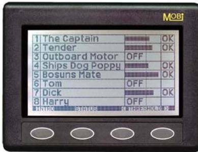
In operation the base station sequentially interrogates each transponder which then broadcasts its presence. In the event of a crew member falling overboard the drop in signal level is detected by the base unit which sounds a high intensity audible alarm.
