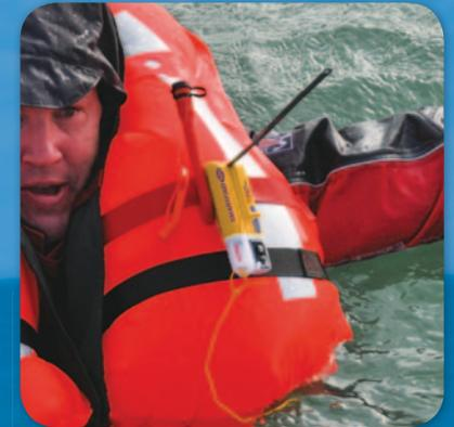
The Smartfind S20 transmits target survivor information, including GPS position information and a serialised identity number back to the onboard plotter. An inbuilt high precision GPS receiver provides accurate position information to assist in quick recovery of survivors.
