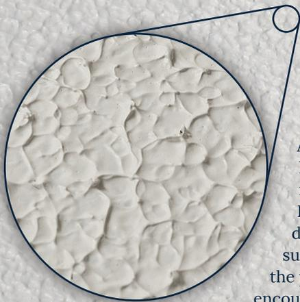
As a homogeneous material, KiwiGrip doesn't suffer from the problems encountered with products filled with sand, walnut shells, beads, rubber fleck, or other fillers. Coatings with fillers tend to wear through, and the fillers fall out leaving an unsafe deck that's hard to clean and even harder to re-coat.
