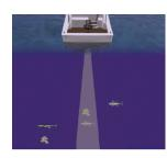
Current high frequency CHIRP transducers have an 8 degree beam width that changes with the frequency.
