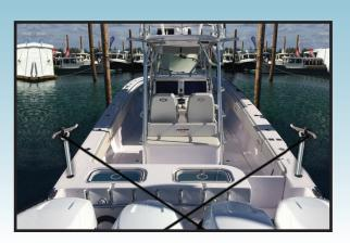
Taco Marine introduces a new Transom Cross Tie device that ensures the ability to get dock lines up and away from outboard motors when tying off at the stern and for motor cowling protection. The patent pending latch mechanism at the base allows easy insertion and hold into standard rod holders. Added features provide multiple use applications in a single, stowable product.
